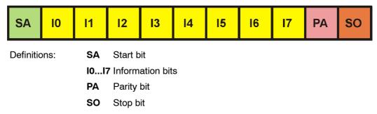
The control characters for procedure 3964R are taken from the DIN 66003 standard for 7-bit code. The transmission itself, however, uses an 8-bit unit interval with bit 7=0. For the purposes of data protection, a block check character (BCC) is sent at the end of each data block.
